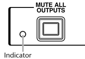
1. On the S-1608 or S-0816 front panel, press and hold the [MUTE ALL OUTPUTS] button. After approximately 1.5 seconds, its indicator will light. No sound is output while the indicator is lit.
