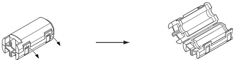
2. Place the REAC cable SC-W100S or Ethernet cable in the ferrite core so that the core abuts the base of the cable's connector.
