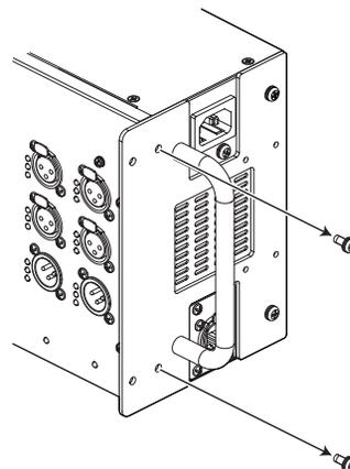
3. Fit the rack mount kit included in the package. Since different mounting brackets are used on the left and right, refer to the diagrams below to select the proper rack ear for each side.
