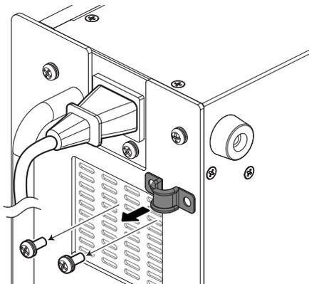
2. As shown in the figure, clamp the AC power cord with the AC Cord Clamp, and secure with the screws (2) removed in Step 1.
