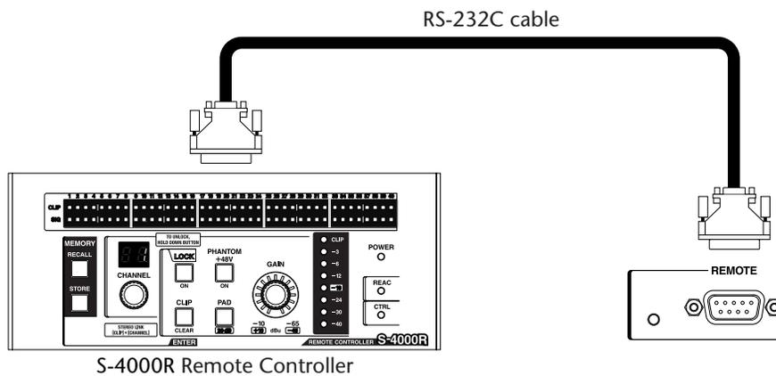
Power is supplied to the S-4000R through the REMOTE connection. The S-4000R's POWER indicator will light when receiving power.
