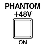
To turn off a channel's phantom power, select the channel with the [CHANNEL] knob, and then press [PHANTOM +48 V] so its indicator goes out.
