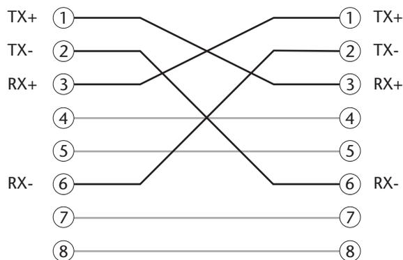
Note: Pins 4, 5, 7, and 8 are not used in this application, but may be wired in the cable as shown.
